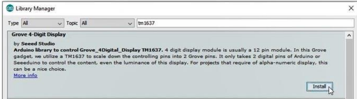
Fig. 5.3 Installing TM1637 library in Arduino UNO
