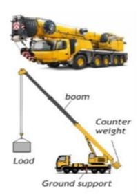
object that is lifted. The counter weight exerts a torque on the crane in equal and opposite direction to the torque from the load. Mathematically,
