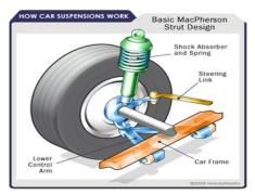
other eye. Any relative motion between the frame and the axle causes the piston to act against the oil in the cylinder. This oil has to leak through small openings or pass through a spring-loaded valve. In this way, a force is created that opposes the contraction and stretching of the springs, and the vibration of the body is dampened.
